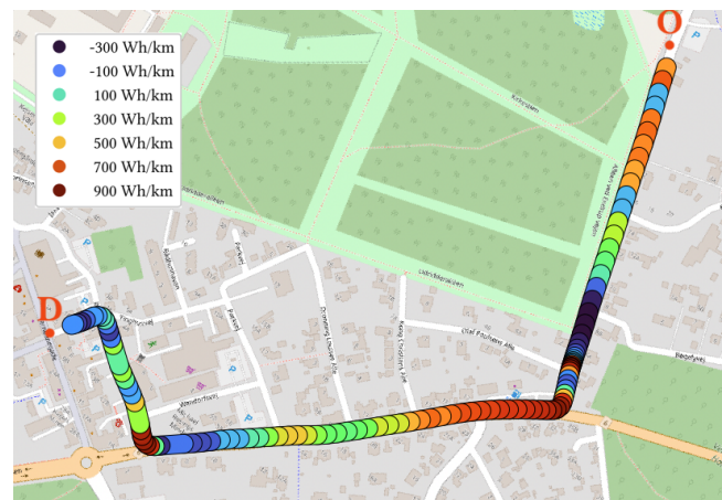
Figure 1: Heat map of the energy consumption of a vehicle during a trajectory.
